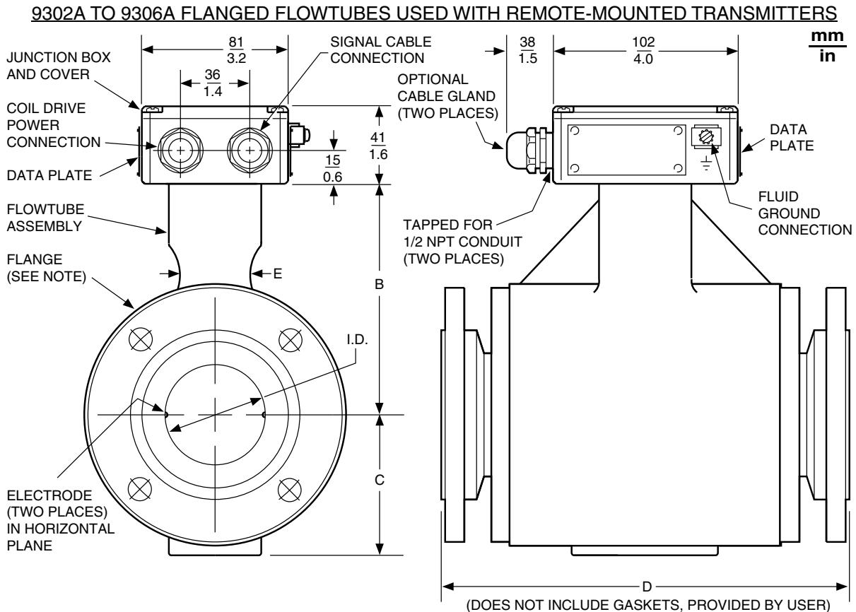
NOTE: Flowtube mounts between the following pipeline flanges: Metric PN 10, PN 16, PN 25, and PN 40; and ANSI Classes 150 and 300.
