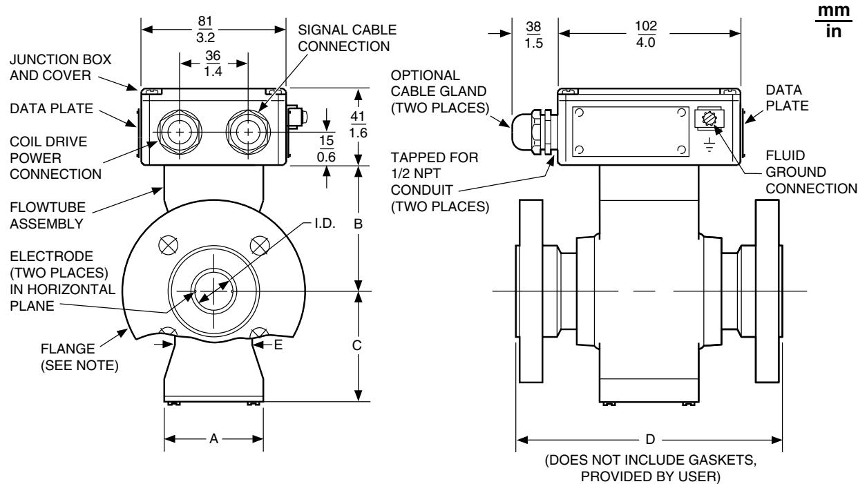
NOTE: Flowtube mounts between the following pipeline flanges: Metric PN 10, PN 16, PN 25, and PN 40; and ANSI Classes 150 and 300.
