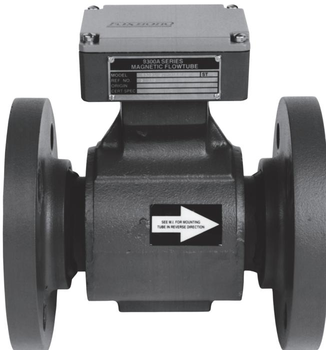
These PFA, PTFE, and polyurethane-lined compact, flanged magnetic flowtubes, together with an IMT25 Magnetic Flow Transmitter combine to form an easy-to-use versatile, dc pulsed Magnetic Flowmeter. The flowmeter measures electrically conductive liquids and produces a measurement signal directly proportional to volumetric flow rate. As symbolized by the CE logo marking on the product, the flowtube conforms to the applicable European Union directives.
