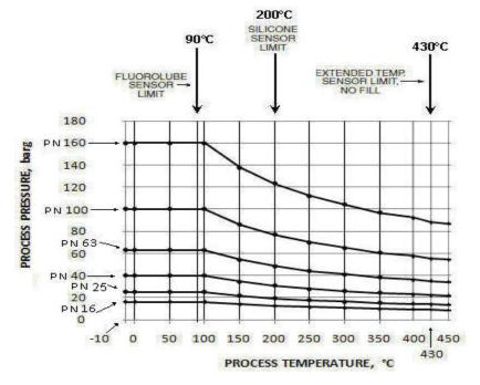
Figure 12. Metric Flange Ratings; per EN 1092-1; Material Group 3E0: Style A: Fabricated Tubes, (DN150 to DN300, 304 SS) and Welded Weld-Neck Flanges (Carbon Steel) Style B: Cast Tubes (DN15 to DN300, CF8M) and Welded Weld-Neck Flanges (Carbon Steel)
