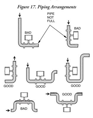
For a clean liquid, the electronics housing can be mounted above or below the flowmeter body. Care should be taken so that entrapped air does not accumulate in the sensor cavity. A meter used on liquid should be mounted upstream from a control valve. Flowmeters can also be mounted with the electronics housing positioned to the side. This ensures escape of entrapped air.
