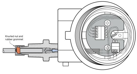
Figure 30. Connection of Remote Signal Cable (Junction Box End)
