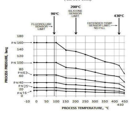
Figure 13. Metric Flange Ratings; per EN 1092-1; Material Group 16E0; Standard Pressure Options: Style B Only: Cast Tubes, DN150 to DN300 Duplex Materials, and Welded Weld-Neck Flanges
