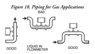
When the process fluid is gas, the electronics housing can be above or below the flowmeter body. The normal recommended position of the electronics housing is above the flowmeter body.
