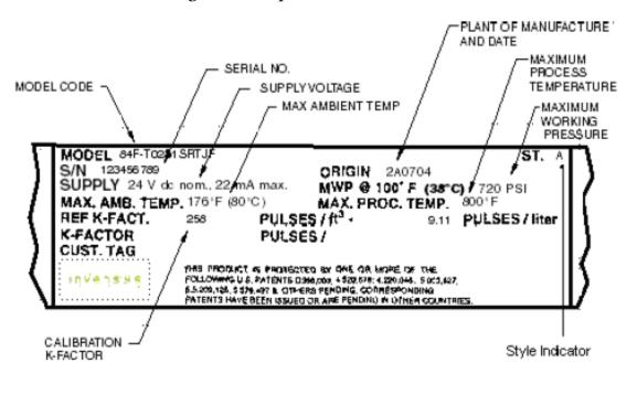
Figure 16. Sample Junction Box Data Plate
