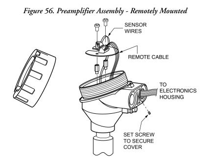
3. Disconnect the (blue-red-orange-yellow) preamplifier wires from the 4-position terminal block and the (yellow and brown) sensor wires from the 2-position terminal block.
