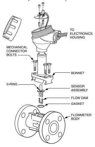
Figure 60. Sensor Replacement - Remotely Mounted Flowmeter
