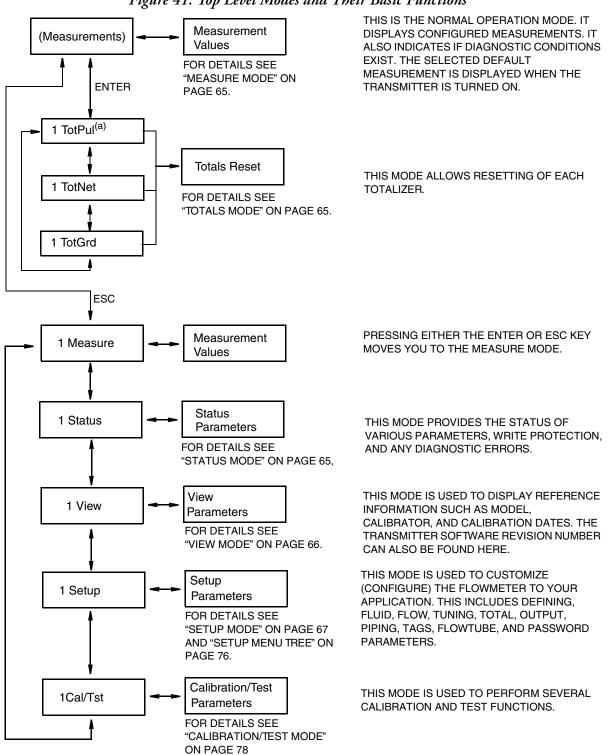
Figure 41. Top Level Modes and Their Basic Functions
