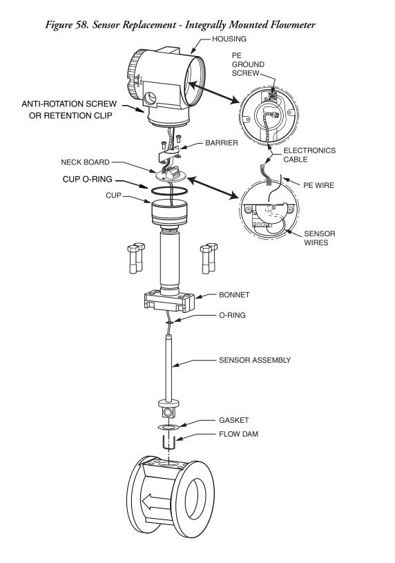
It is important that the gasket be sealed uniformly to provide a good seal. The following two steps assure a uniform seal. Failure to follow these steps could result in personal injury due to gasket leakage.
