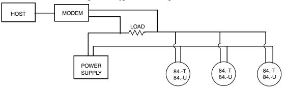
The HART Communicator can operate, configure, and calibrate 84 Series Flowmeters with HART communication protocol in the same way as it can in a standard point-to-point installation.
