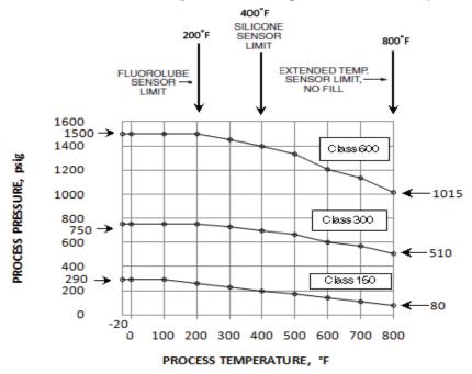
Figure 9. ANSI Flange Ratings; per ASME B16.5; Group 3.8 Materials; High Pressure Options: Style B Only: Cast Tubes (3/4 to 8 Inch, CX2MW Nickel Alloy [equivalent to Hastelloy® C-22]), and Welded Weld-Neck Flanges (N06022 [equivalent to Hastelloy® C-22])
