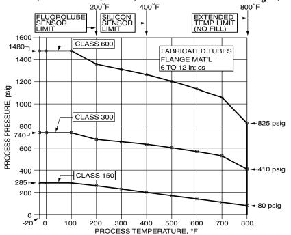
Figure 5. ANSI Flange Ratings; per ASME B16.5; Group 1.1 Materials; High Pressure Options: Style B Only: Cast Tubes (3/4 to 8 Inch, CF8M), and Welded Weld-Neck Flanges (Carbon Steel)
