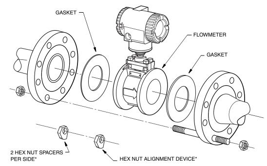
Figure 25. 84W Flowmeter Centering (using Spacers)
