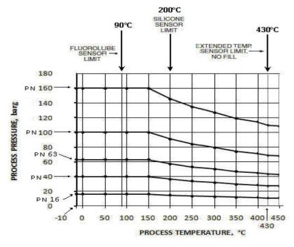
Figure 11. Metric Flange Ratings; per EN 1092-1; Material Group 10E0s: Style A: Fabricated Tubes (DN150 to DN300, 304 SS) and Welded Weld-Neck Flanges (304 SS) Style B: Cast Tubes (DN150 to DN300, CF8M) and Welded Weld-Neck Flanges (304 SS)
