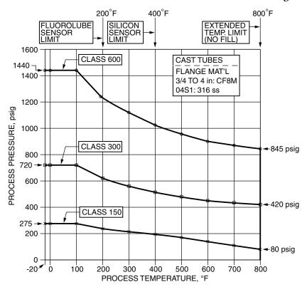
Figure 2. ANSI Flange Ratings; per ASME B16.5; Group 2.2 Materials; High Pressure Options: Style B Only: Cast Tubes (3/4 to 4 Inch, CF8M) and Welded Weld-Neck Flanges (316 SS)
