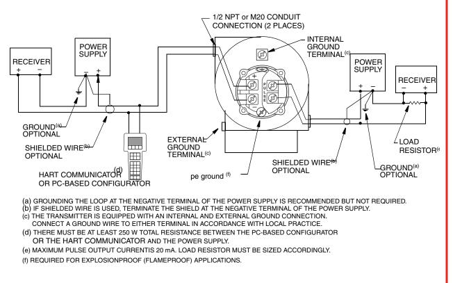
Figure 38. Wiring an 84F-T (Styles A and B) or 84W-T Flowmeter with a Pulse Output Transistor Switch (sourcing) Counter Input with External Power Supply and Pull-Up Resistor
