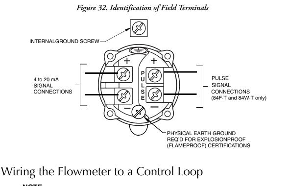
When wiring a flowmeter with 4 to 20 mA output signal, the supply voltage and loop load must be within specified limits. The supply output load vs. voltage relationship is shown in Figure 33.
