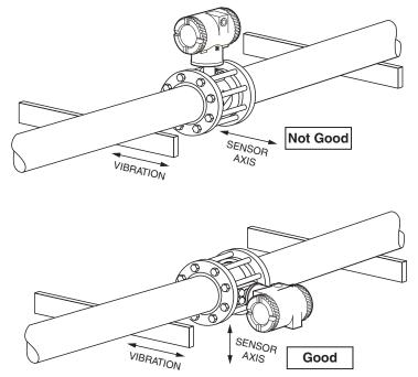
Figure 21. Sensor Mounting to Minimize Effect of Vibration
