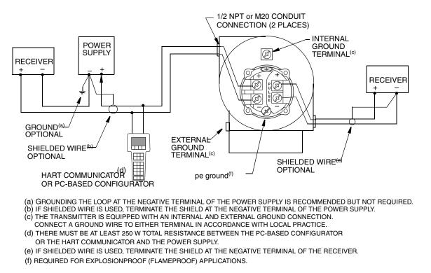
Figure 37. Wiring an 84F-T (Styles A and B) or 84W-T Flowmeter with a Pulse Output Transistor Switch (sinking) Counter Input with External Power Supply and Pull-Up Resistor
