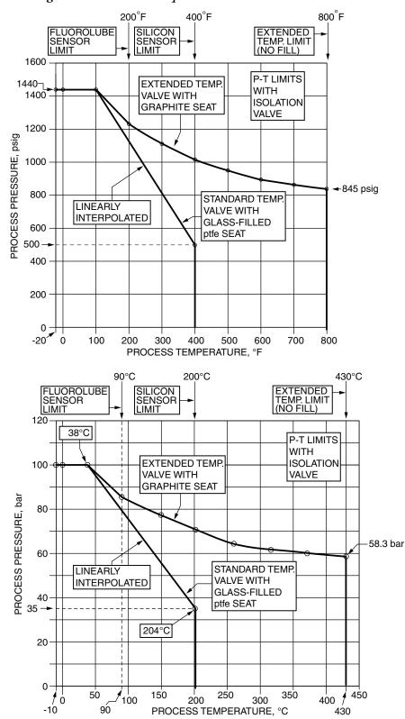
Figure 14. Pressure - Temperature Limits with Isolation Valves
