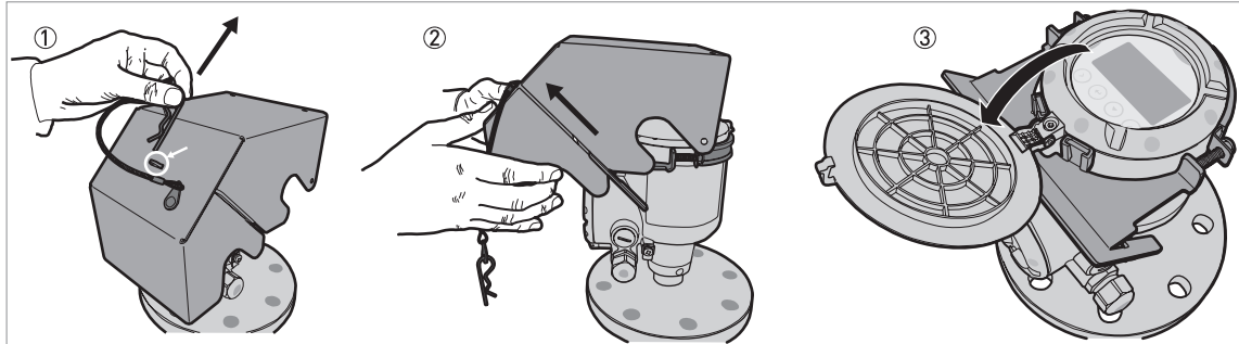
Figure 3-26: How to open the weather protection
