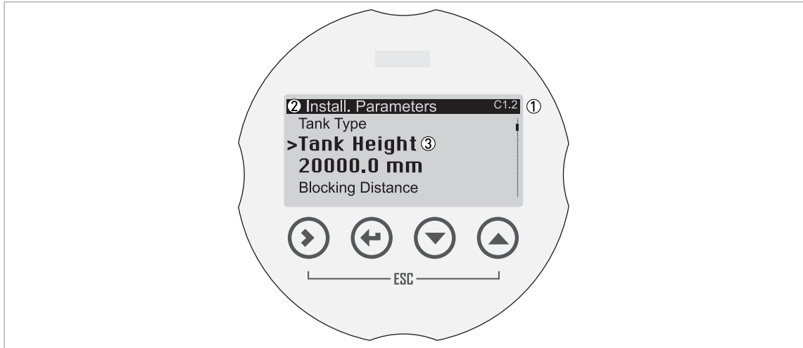
Figure 5-2: Display screen layout in Program mode
