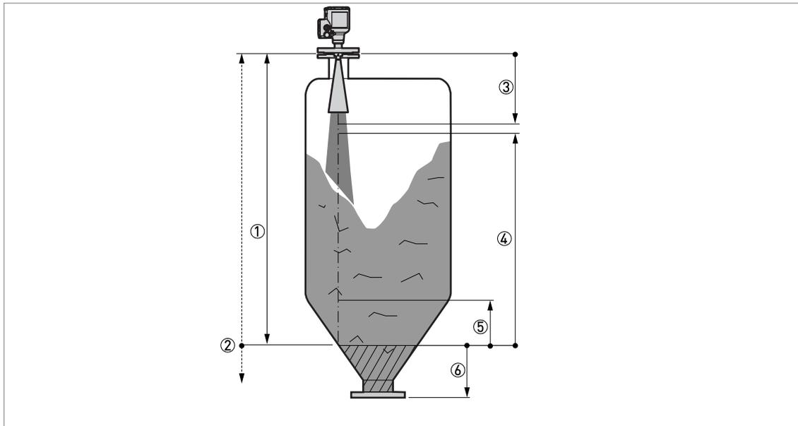
Figure 6-8: Level measurement
