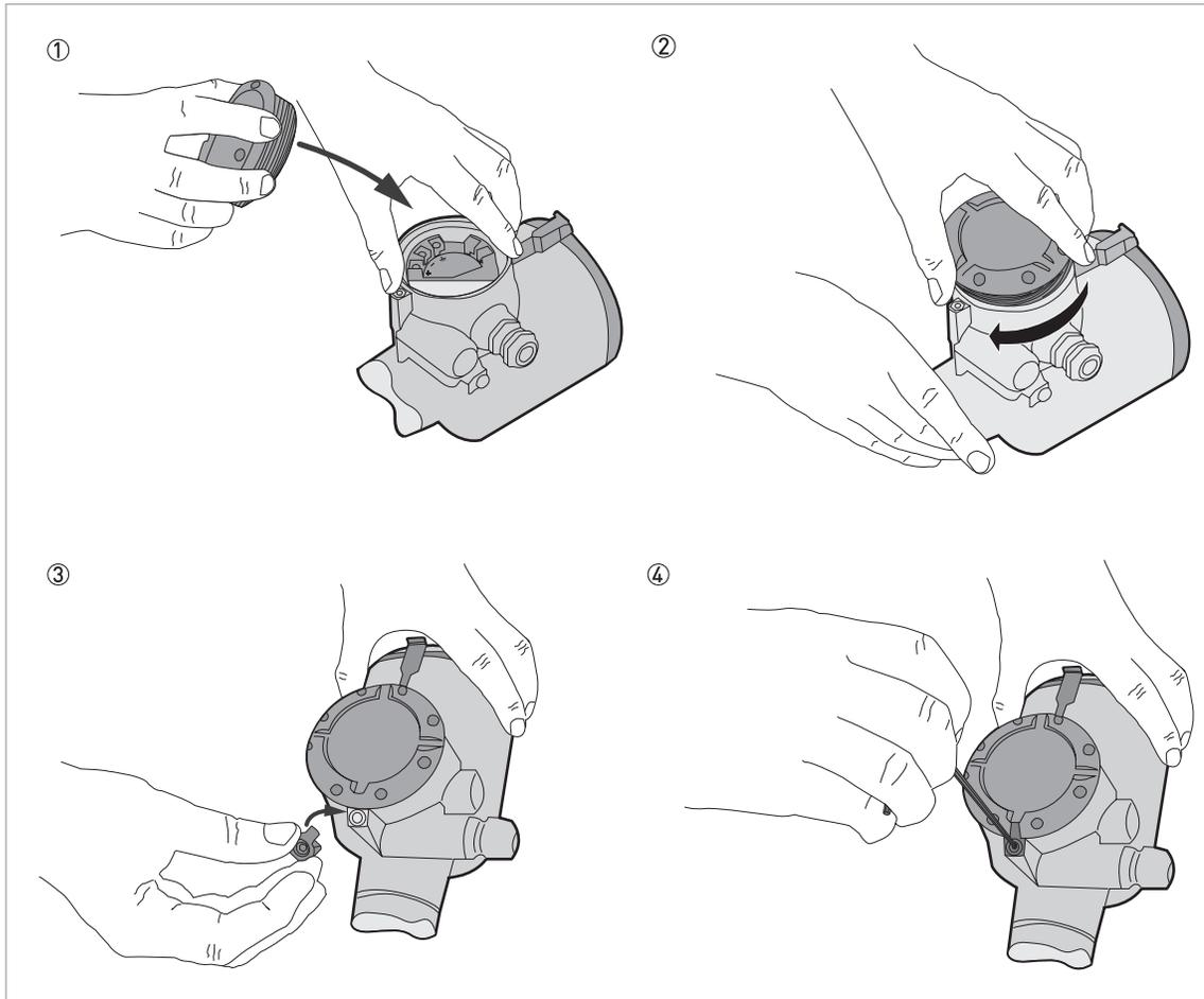
Figure 4-4: How to close the terminal compartment cover
