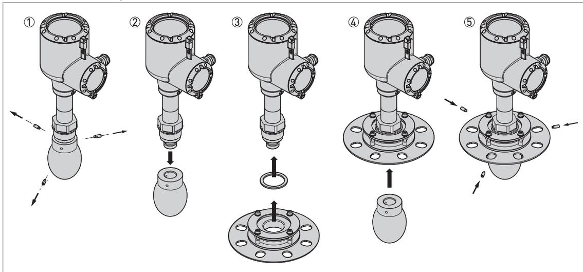
Figure 3-17: Device with a Drop antenna
