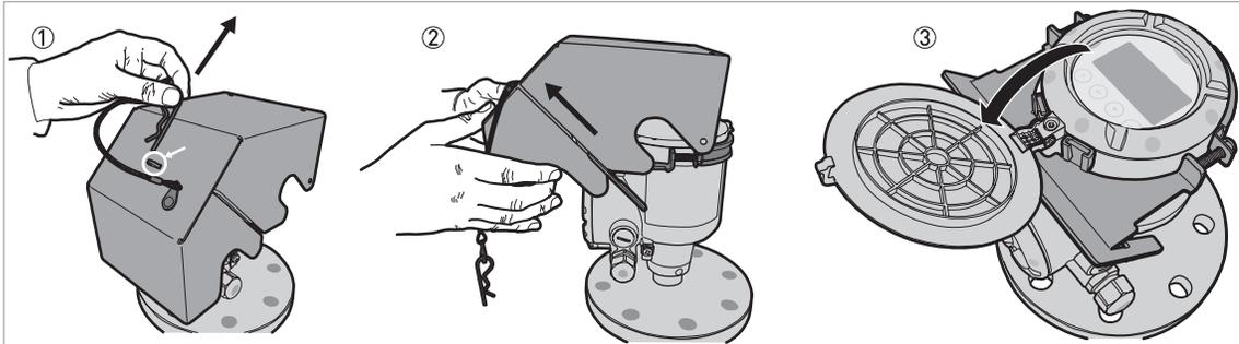
Figure 3-22: How to open the weather protection
