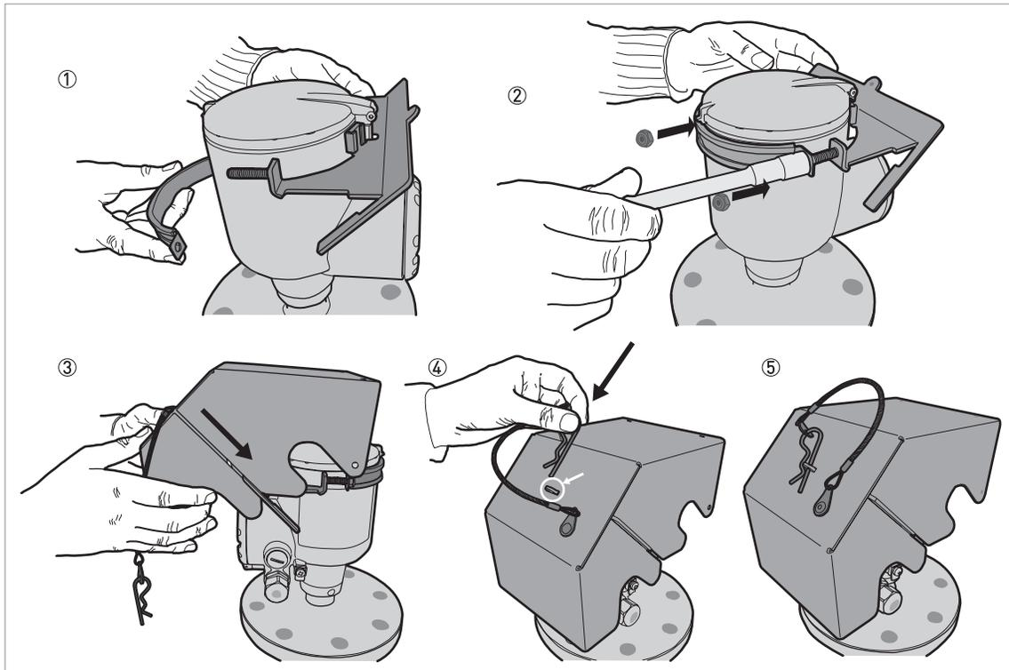
Figure 3-21: Installation of the weather protection
