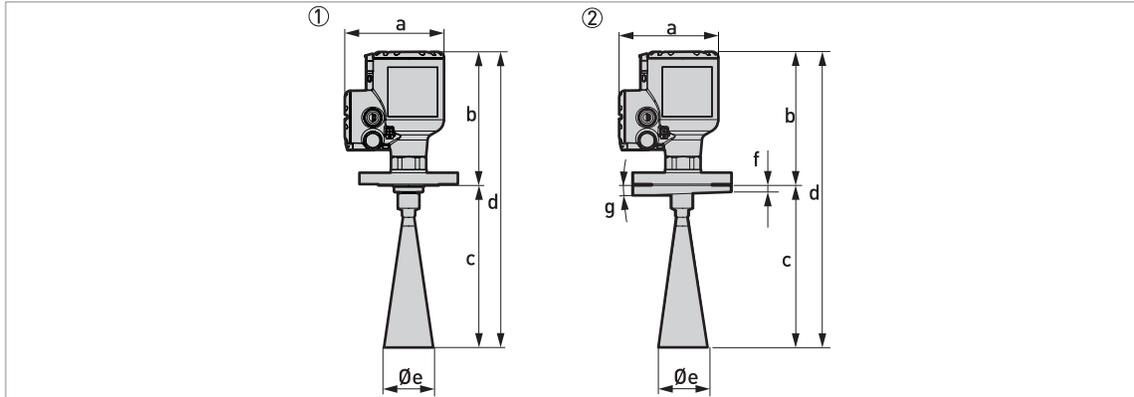
Figure 8-11: Metallic Horn antennas with standard flange connections
