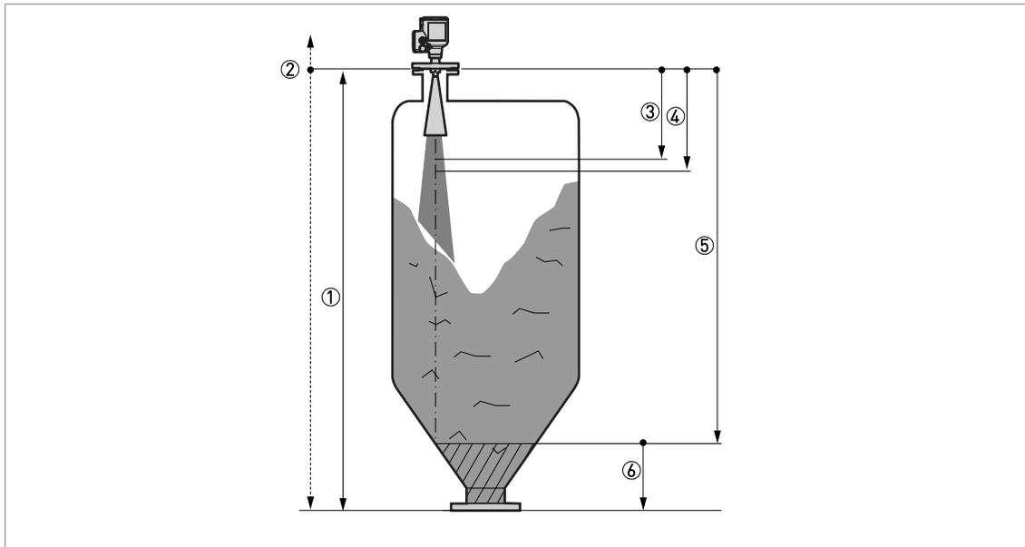
Figure 6-7: Distance measurement
