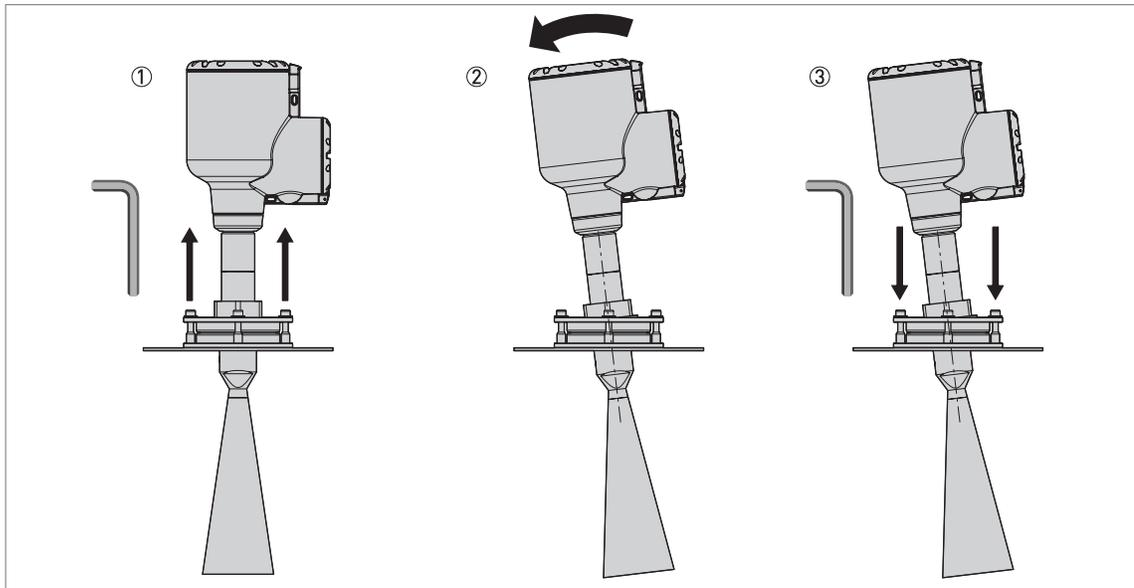
Figure 3-18: How to tilt the device
