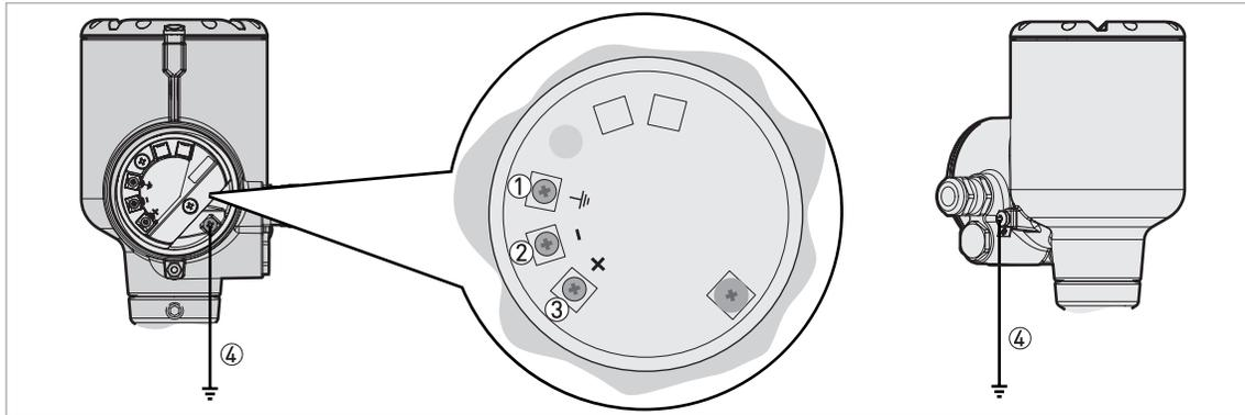
Figure 4-1: Terminals for electrical installation: standard cable gland
