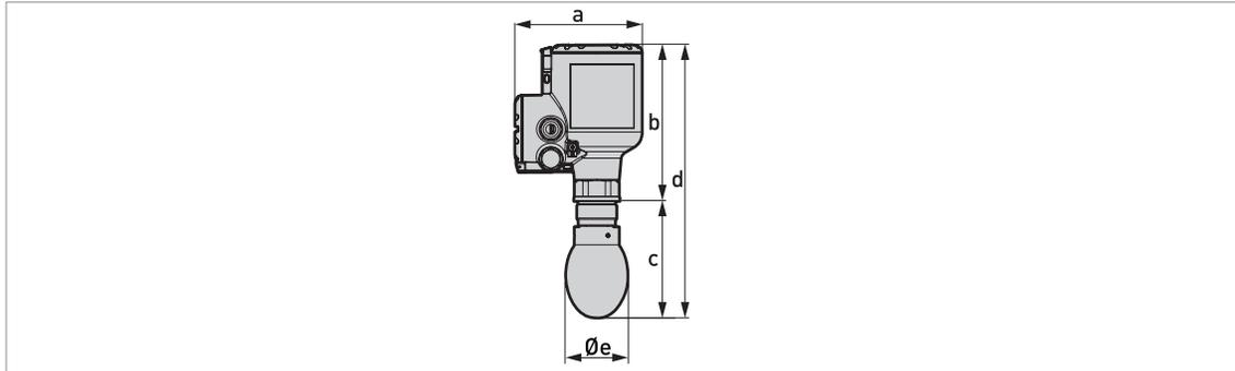
Figure 8-13: Drop antennas with threaded connections
