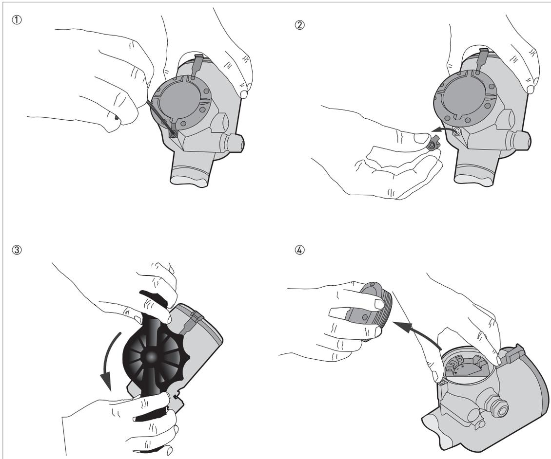
Figure 4-2: How to open the terminal compartment cover
