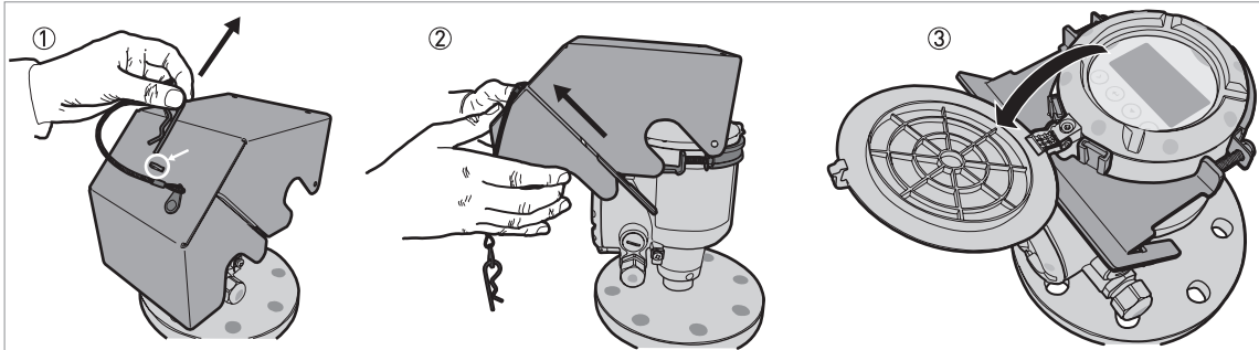
Figure 3-25: How to open the weather protection
