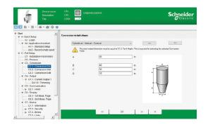
A conversion table can be entered through the display or with the PACTWare DTM (shown above) to allow volume output based on standard or custom tank shapes. Volume, ullage volume, mass and ullage mass are all available as measurements. Users can select from standard units of measurement or create their own as a custom option.
