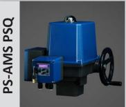
Torque: 130 - 1.000 Nm Operation Time: 9 - 140 s for 90° Enclosure: IP67 or IP68 according to DIN EN 60529 Valid ambient temperature: -20 to +60°C
