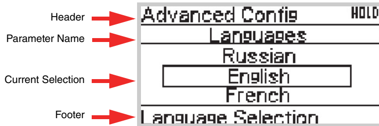
Figure 19. Four Lines Can Be Scrolled if the Screen Includes a Parameter Name and a List of Selections
