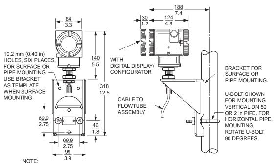
WHEN THE BRACKET IS USED FOR WALL MOUNTING, REPLACE U-BOLT WITH TWO (OR FOUR IF NECESSARY) 0.375 IN BOLTS OF SUFFICIENT LENGTH TO PASS THROUGH THE BRACKET AND SURFACE
