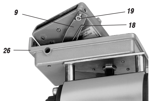
Fig. 23: Attachment of the positioner
