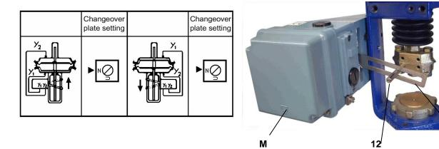
ensure that the feedback lever 11 is horizontal at 50 % stroke.
