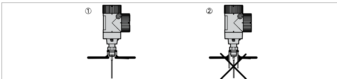
Figure 3-4: Sockets for threaded process connections
